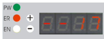
Figure 15 : Example of Error message at the 7-segment display
