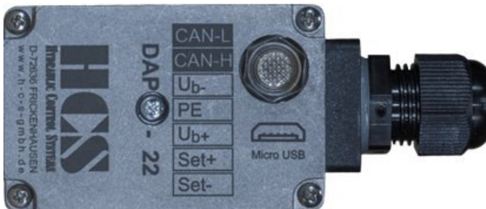
Figure 2 : Top view onto unit
