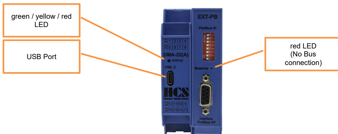
Figure 10: Top view, status LEDs and USB Port
